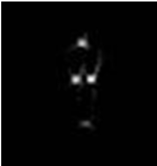
Figure 5. Reconstruction of four point sources with varying intensities, created by applying a different number of exposures at each point.
