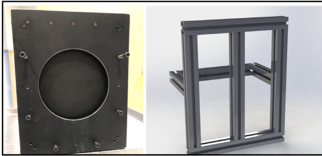
Figure 4. Left: The TR camera with a 15 cm diameter aperture, and the CR plate a few centimeters back from the aperture. The screws are in place in order to attenuate x-rays which could enter through holes that had been drilled into the camera face to accommodate a previous design. Right: The aluminum frame which supported the CR plate.
