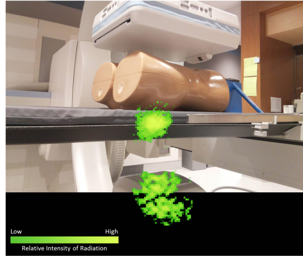
Figure 8. An x-ray scatter reconstruction (seen in figure 7) overlaid with the photograph of the scene. X-ray scatter is shown in green.
